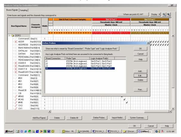
Note: In the above picture under Logic analyzer pods, the first pod goes to the Odd pod and the second goes to the Even pod of the termination adapter (e.g. Pod B1 goes to odd termination adapter pod and B2 goes to the even termination adapter pod).
